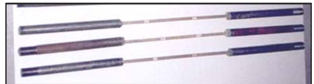
Figure 1: Preparation of GFRP bars specimens
